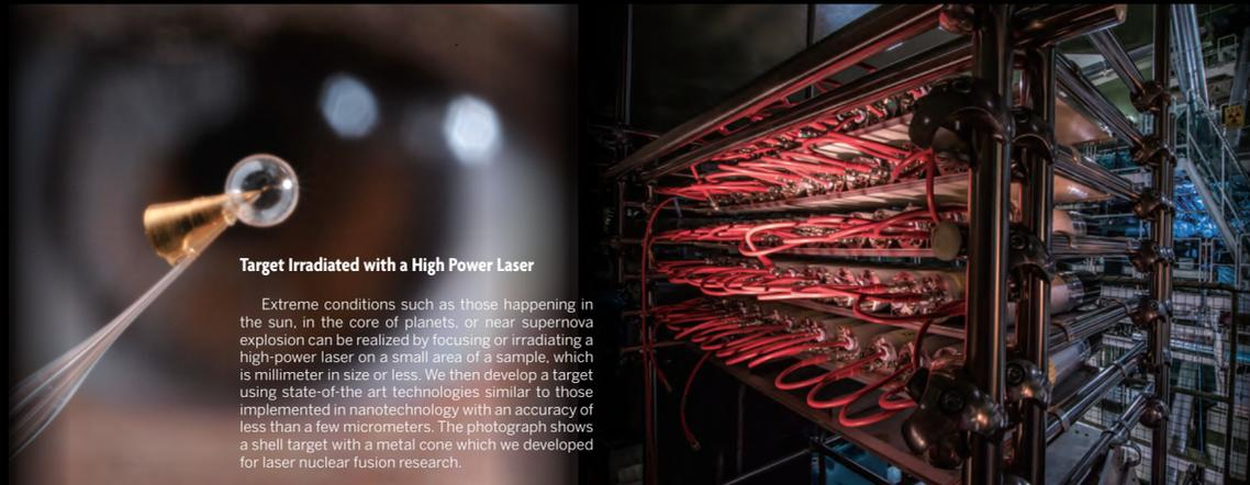
**Target Irradiated with a High Power Laser**
