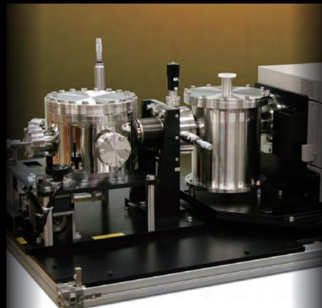
◀ **Ultrahigh-speed Camera for Vacuum Ultraviolet Spectroscopy**
