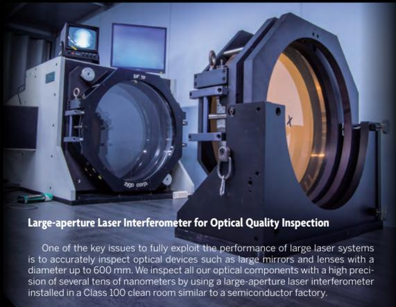
**Large-aperture Laser Interferometer for Optical Quality Inspection**
