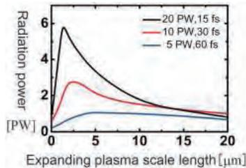
Fig. 1 Gamma-ray power dependence on laser and plasma parameters. Three lines correspond to different laser power with a fixed laser energy ( $E_L=300\text{J}$ ). There exists an optimum scale length for the effective gamma-ray generation.
