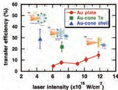
Figure 1: The transfer efficiency as a function of the laser intensity for three targets.
