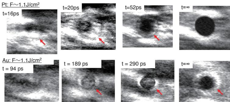
Figure 1 : The time-evolution of the soft x-ray reflectivity after the femtosecond laser irradiation on Platinum (Pt) and gold (Au).
