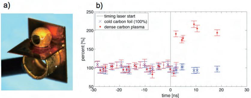
Figure 1: a) Double hohlraum target. b) Energy loss measurement in a cold carbon and a plasma
