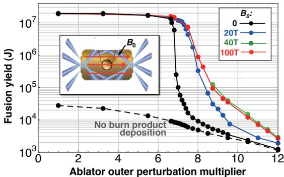
Figure 1: Fusion yield of the NIF cryo-DT ignition target versus multiplier on the amplitude of capsule outer surface perturbation under initial seed magnetic fields from 0 to 100 T [1].
