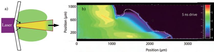
Figure 1 (a) Schematic of an irradiated cone target that produces a collimated jet. (b) Density distribution of a collimated jet calculated by the radiation-hydrodynamic code CRASH for a 100- $\mu\text{m}$ -thick plastic cone target irradiated by a 5 ns drive pulse. The color scheme is on a log-scale for fluid densities ranging from  $10^0$ - $10^{-4}$   $\text{g}/\text{cm}^3$  and illustrates the radial and axial variation in the jet density.
