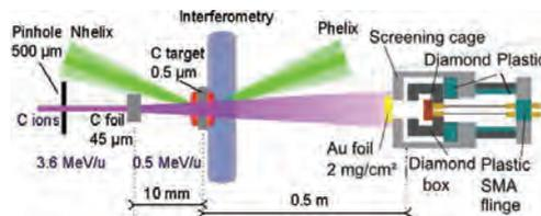
**Fig.1:** Experimental setup for the energy loss measurement at stopping maximum in plasma
