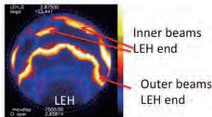
Figure 2: Time-integrated image looking into OPEN end at 180 to hohlraum axis at x-ray band of 3-5 keV
