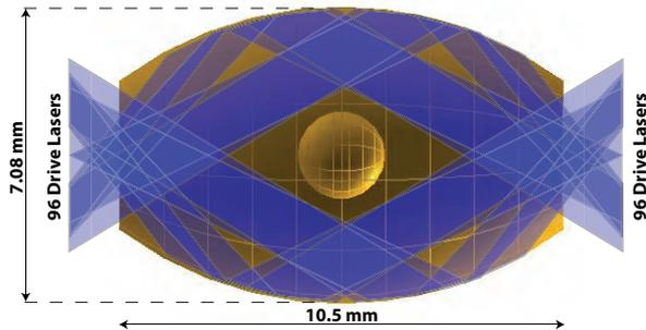
Figure 1: The rugby-shaped hohlraum heated with a total of 192 NIF laser beams.
