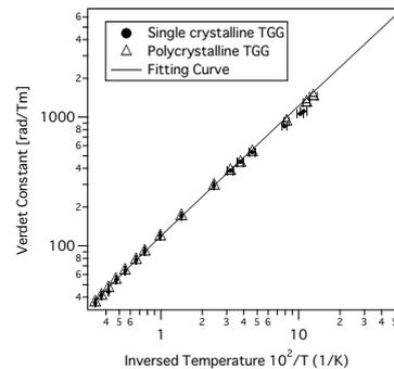
Fig. 2. The temperature dependence of Verdet constant of single crystal and TGG ceramic.
