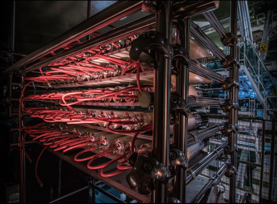
◀ MANDALA : Multi-channel Detector of Neutrons from Nuclear Fusion Reactions
