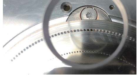
Figure 2: Disk rotor with 200 large holes(upper in figure) rotates at 20 s period. Lower small holes are for monitoring the injection timing.
