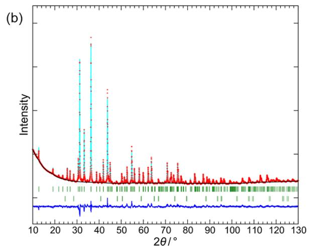
Figure 1. Results of the Rietveld analysis of Sr<sub>3</sub>Sc<sub>2</sub>Ag<sub>2</sub>Se<sub>2</sub>O<sub>5</sub>. Red points represent the experimental patterns, cyan line the calculated patterns, and blue line the difference of these patterns.
