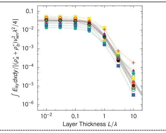
FIG. Dependence of the integrated kinetic energy measured at the nonlinear regime on the thickness of the transition layer L. Various parameter runs are plotted with different marks. The gray thick curve is the fitted function of all the data, which are proportional to  $[1 + (qL/\lambda)p]^{-1}$  with q = 2.11 and p = 2.46.
