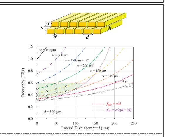
FIG. A schematic illustration of the two-tier metallic slit-array structure and the critical frequencies,  $f_c$ , shown for various slit widths, w, as functions of the lateral displacement, l. The  $f_c$  can actually be found only in the region colored yellow-green.
