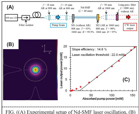
FIG. ((A) Experimental setup of Nd-SMF laser oscillation, (B) Fluorescent beam profile image of Nd-SMF output, the beam quality factor is M<sup>2</sup>=1.0, (C) Input-output characteristics of Nd-SMF laser) Lateral displacement effects on the optical transmission properties of stacked metallic sub-wavelength slit-array systems Y. Tokuda<sup>1,2</sup>, K. Sakaguchi<sup>1</sup>, S. Watanabe<sup>1</sup>, M. Nakajima<sup>2</sup>
