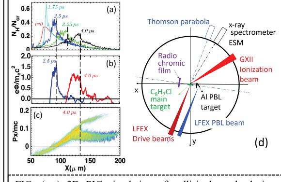
FIG. (a-c) 2D PIC simulation of collisionless shock ion acceleration. Temporal evolution of (a) proton density, (b) electrostatic potential, and (c) proton phase-space. (d) Top view of the experimental setup.
