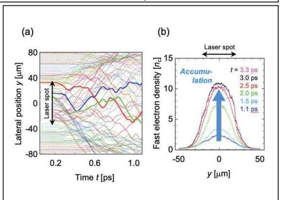
FIG. 2D PIC simulation for the continuous irradiation of a laser with amplitude  $a_0 = 1.4$  and spot radius w ((a)  $w = 35 \,\mu\text{m}$ , (b)  $w = 21 \,\mu\text{m}$ ) onto a 5  $\mu$ m-thick, 100  $n_c$  foil plasma. (a) Fast electron trajectories exhibiting a random walk in the lateral direction. (b) Fast electron density accumulated in the foil.
