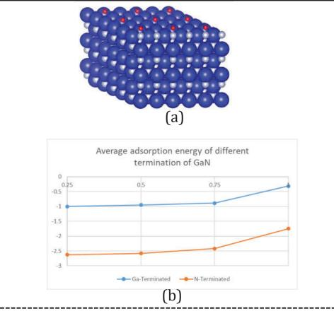
FIG. 1 (a) Optimized configuration of the N-terminated GaN (100) surface with 0.25 ML adsorbed H and (b) average adsorption energies of adsorbed H at different coverages on both Ga- and N-terminated GaN (001) surfaces.
