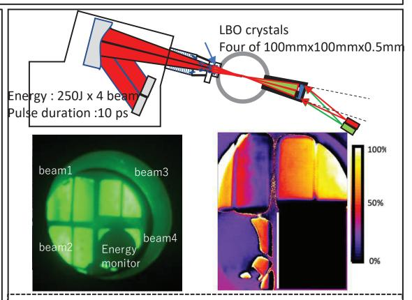
FIG1.(Top) Experimental setup. FIG2. (Left bottom) Color image of the second harmonics beam patterns for four beams. FIG3. (Right bottom) Spatial profile of the frequency conversion efficiency. Beam2 was blocked by energy monitor beam 4 was not fired in the shot.
