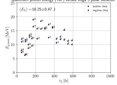
Fig. 1: Example of a dataset obtained for fixed pulse energy, spot size and target thickness while varying the pulse duration from 30 to 600 fs. It appears clear the non linear dependence of the accelerated ion energy to the pulse duration, in direct contrast to most existing scaling laws.
