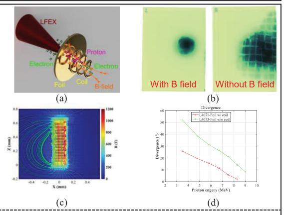
FIG. (a) The schematic of the experiments. (b) Proton pattern of 4.8 MeV on RCF. (c) The 2D B field strength distribution around the coil. 1-kT strong B field is generated with a laser energy of 334.3 J. (d) Comparison of the proton divergence with B field (red) and without B filed (green).
