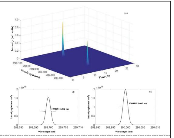
FIG. Three-dimensional spectral and temporal profiles of the two emission wavelengths from a double Littman resonator. Spectral profile of the two emission wavelengths. The linewidth of both emissions is 2 pm.
